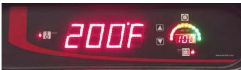
**DISPLAY...** Bright LED digital temperature and battery charge display for easy viewing from a distance. Adjustable brightness for indoor or outdoor viewing.
