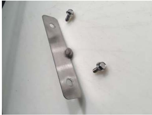
2. Remove the door latch and reinstall the latch in the location where the door latch trim plate was just removed.
