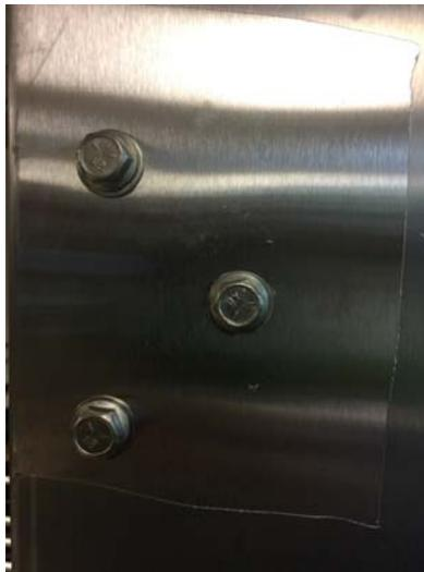
11. With assistance, remove the (6) bolts that attach the door hinges to the cabinet. There are (3) on the top and (3) are the bottom.
