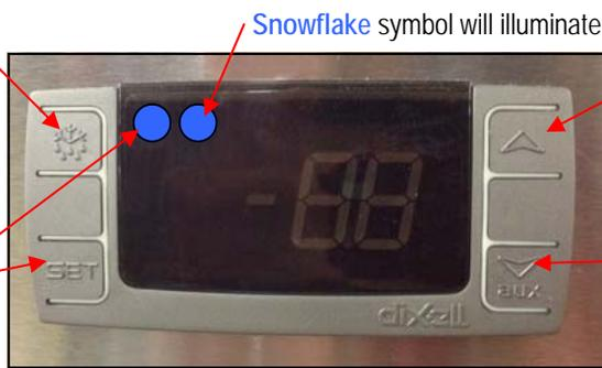
**Snowflake** symbol will illuminate here when compressor is ON
