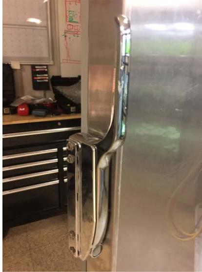
10. Remove the (6) bolts, (3) for the top, (3) for the bottom, located on the side of the cabinet opposite from the door hinges and set aside.
