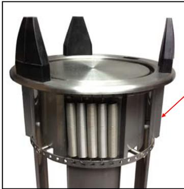
Lift entire tube out of cabinet to adjust springs
