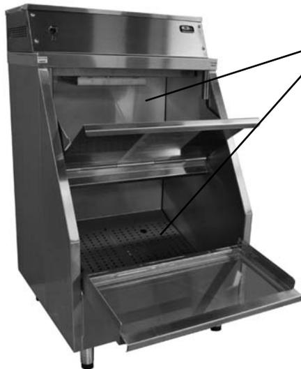
**EXCLUSIVE HEAT DUCT BAFFLING SYSTEM...** Warm air is directed through duct in back of cabinet and up through chips on the bottom. Assures uniform temperatures throughout cabinet for consistent holding of product.
